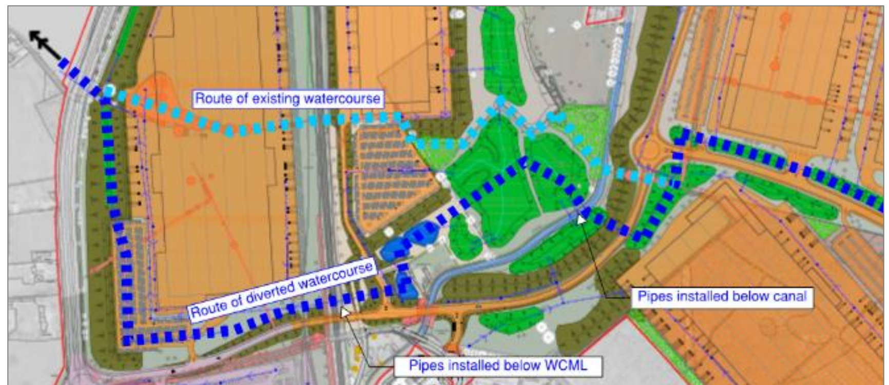
Figure 72: Land drainage ditch diversion
